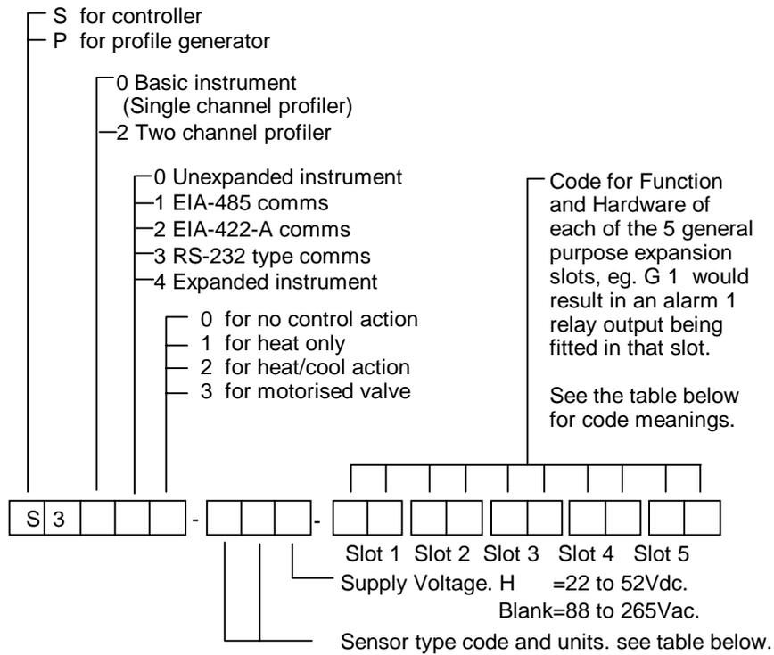
Example 1. S3001-03-B4 G1 This describes an unexpanded controller, with a heat only analogue 0 - 20 mA control (in slot 1), and one alarm of relay type in slot 2. the instrument will be delivered configured for a type K thermocouple and work in degrees C. The 0 - 20mA control output may be set by the user in software, to have a live zero, for example, 4 - 20mA.
