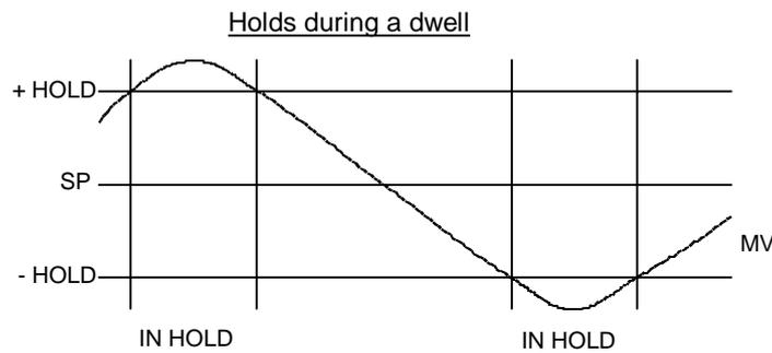
Dwell timer suspended during hold. Note that 'Above', 'Below' and 'Dwell' holds at least are set on in the hold-type parameter of the programmer long scroll.
