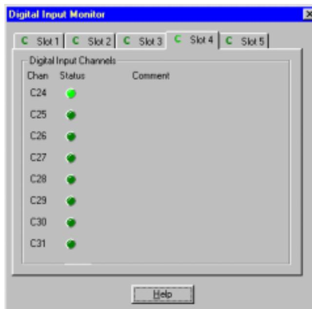
This box is used to monitor the current status of the digital inputs connected to the ICU.
