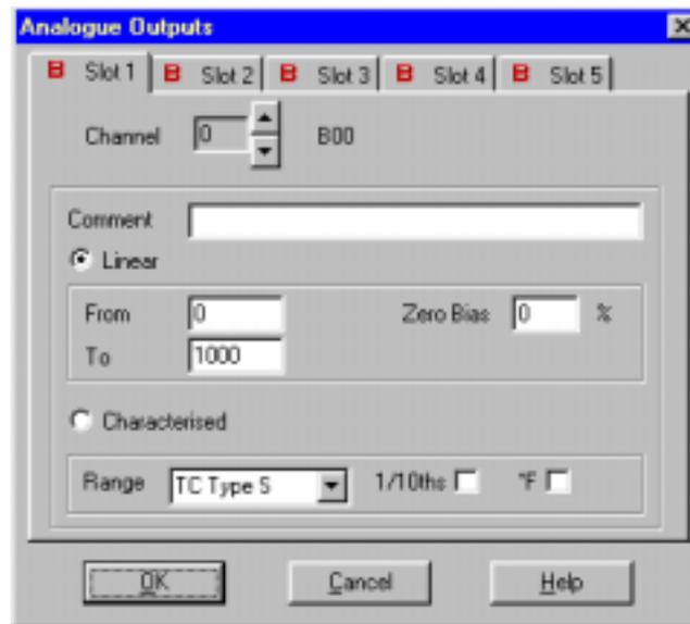
An analog output can work in one of two modes. Select the required mode for the output by clicking the **Linear** or **Characterised** radio button.
